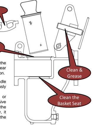
7.7.5 Examine O-Ring mating surface on the underside of the filter cover and ensure that it is perfectly clean, lightly smear the area with grease\*\* and lower the cover onto the filter body.
